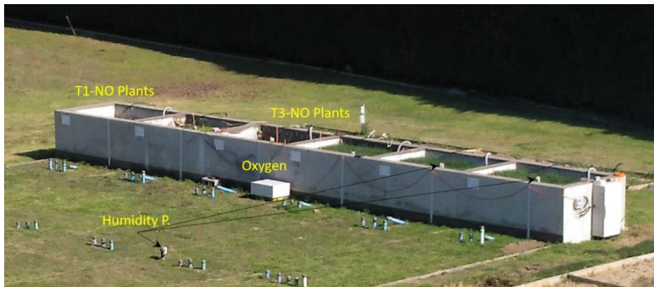
Figure 2: General view of recharge basins and aquifers (6). T1 and T3 are the NO plants representative basins. Oxygen probes are installed at T2, T3 and T4 systems at 5, 10, 15 and 20 cm from surface. Humidity sensors are placed in the middle of the basin surface and in the T5 aquifer close to B piezometer section.
