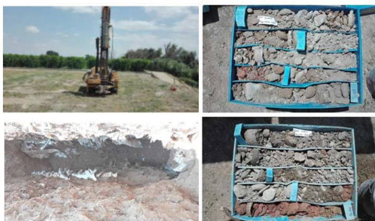
Figure 6: Image of the area selected for the implementation of the MAR prototype (left) and detail of the stratus found (right) shown a very high heterogeneity.
